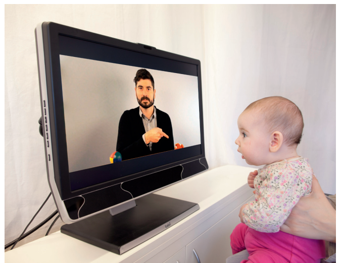
Eye tracking technology is for instance used in infant behavior research. Using an eye tracker you can exactly see where the child is looking. In this picture an eye tracker from Tobii is used.
