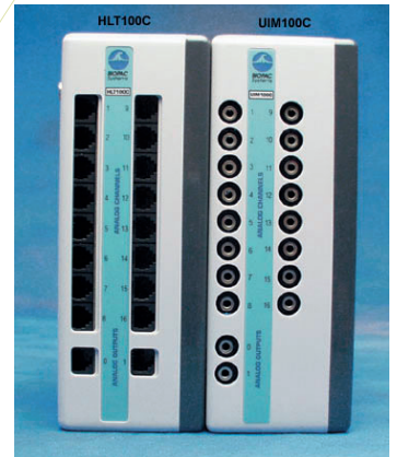
A multi channel stationary DAQ unit.
